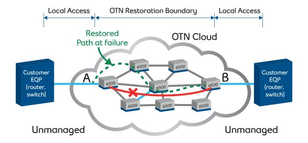
In short, this approach provides users with a double layer of protection: if the working route fails, traffic shifts over to the protection route. If that route fails, it moves over to the dynamically calculated restoration path. In this way, mesh restoration provides a clear advantage over non-OTN static restoration, where a fault in the secondary path would result in a total service outage for the end user.
