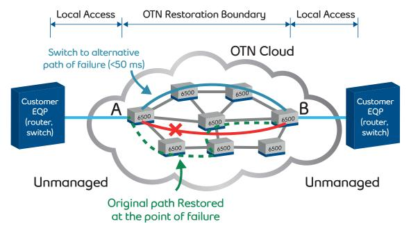
Restoration of the failed circuit will continue until the original working route has been repaired. Without OTN-enabled restoration, the customer's service would remain completely down until the original outage is repaired.
