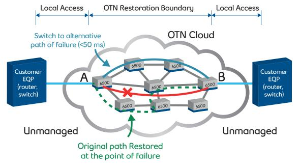
Restoration of the failed circuit will continue until the original working route has been repaired. Without OTN-enabled restoration, the customer's service would remain completely down until the original outage is repaired.
